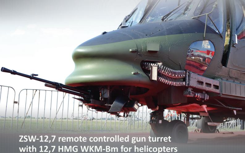
The ZSW-12,7 is designed for arming helicopters and other aircraft with integral on-board remote-controlled weapons system, including the use of helmet systems of helicopter
